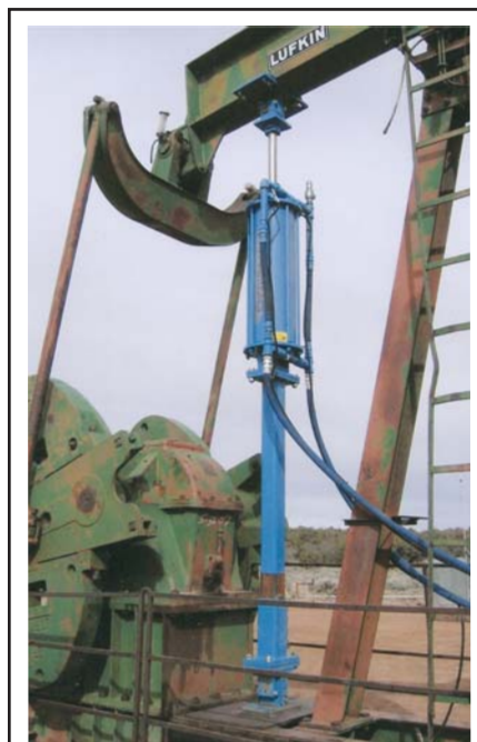
Shown here is one of the beam-operated gas compressor installations at CrownQuest Operating's Apache Jicarilla Field in the San Juan Basin.
