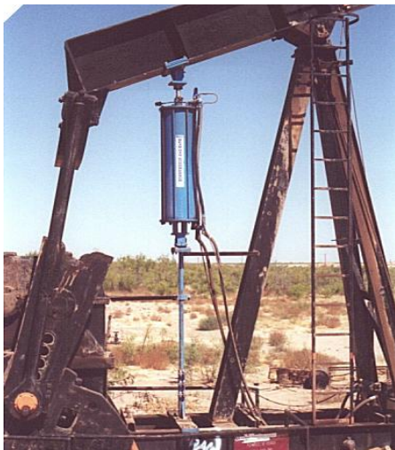
Beam Gas Compressor™ Installation
